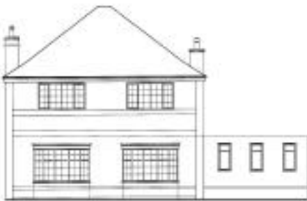
Sketch showing inappropriate flat roofed extension
