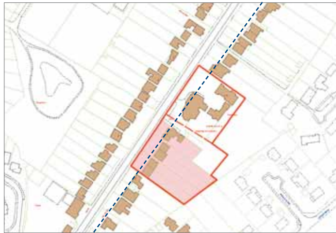
A location plan with the site hatched in red and the building line clearly indicated as a blue dotted line
