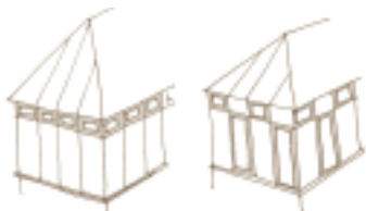
Weak looking frames, flimsy plastic claddings, clumsy vents and haphazard openings
