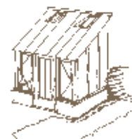
A simple lean-to roof that doesn't project too far...and a pitch that isn't too shallow
