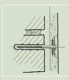
Head of screw is sunken beneath the finished surface of the new plaster
