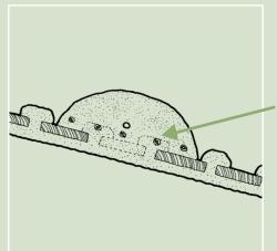
The Plaster of Paris mix is laid over the void left by the removal of the failed lath
