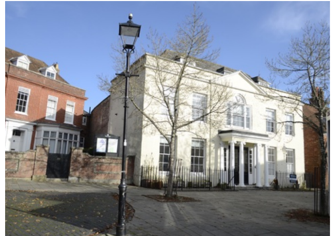
Figure 53: The Old Bank House, is a building of great historic significance faced with yellow mathematical tiles, which are tiles fitted together to look like bricks.
